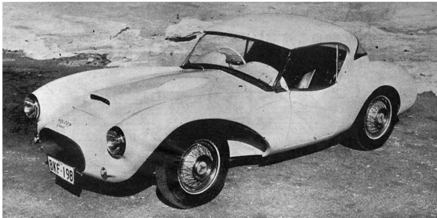
Dummy wire spokes have been added to car to relieve bulk of disc wheels. Bulge on bonnet top is functional.
