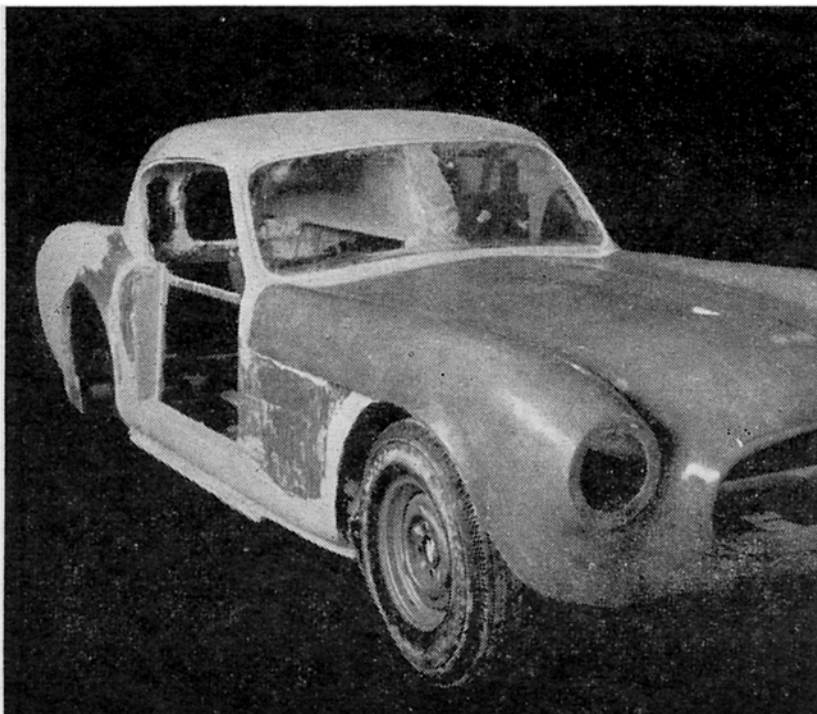
The plaster mould for the Buckle car, with the completed fibreglass bonnet added to show the lines.
