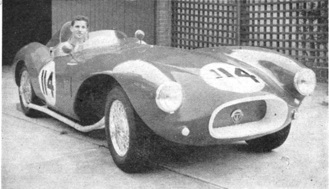
Although basically Buchanan body, the Gladiator's shell is much modified, includes headrest for driver. Fibreglass is only half normal thickness.
