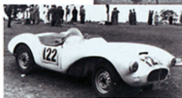
From top: Cobra; TD-based racer won NSW events such as hillclimbs; 16in wires possibly ex-Riley, finned drums; driver sits high, exposed to elements; body moulded off DB3S
