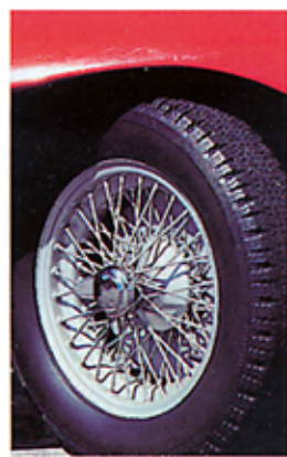
From top: Cobra; TD-based racer won NSW events such as hillclimbs; 16in wires possibly ex-Riley, finned drums; driver sits high, exposed to elements; body moulded off DB3S
